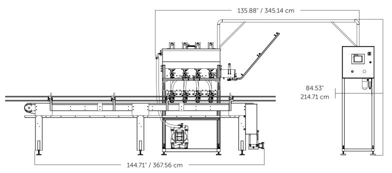
\*ABE's TruPatriot is not complianced as an "explosion-proof filling system". Use equipment in a well-ventilated area to reduce flammable conditions. The operator should ensure that products to be filled do not contain elevated alcohol levels that would otherwise be volatile and/or flammable.
